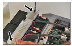
1 Remove the two Phillips screws on the retaining bracket and lift the bracket off.
